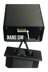
The device is intended for listening to conversations from a room over very long distances. The device operates on the principle of 4G GSM network, and for its normal operation it is necessary to ensure a normall SIM card. The location where the device will operate must be covered by a GSM signal (check with a regular cell phone).
